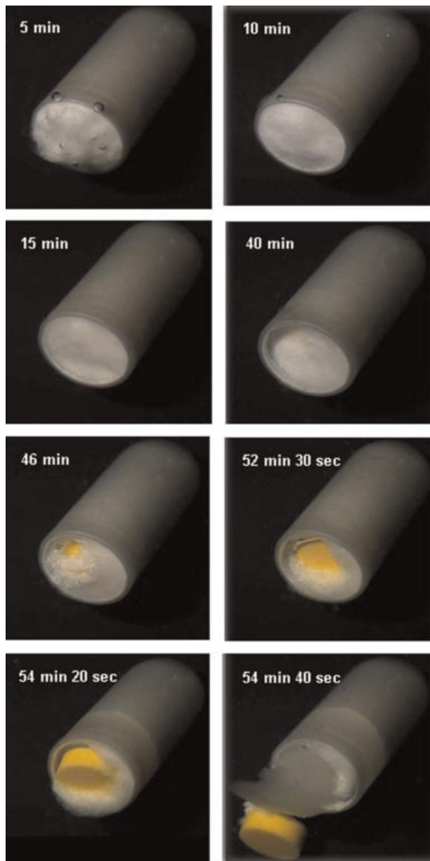
**Figure 2.** The process of pulsed release drug delivery from a TDC fitted with an 80 mg 15% hypromellose ET showing release of a riboflavin tablet.
