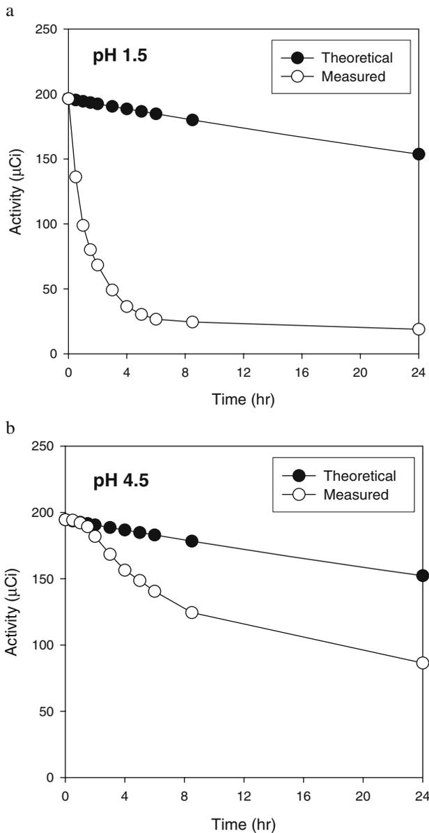
**Fig. 2.** a Dissolution at pH 1.5 of a GRF with <sup>153</sup>Samarium Oxide powder. b Dissolution at pH 4.5 of a GRF with <sup>153</sup>Samarium Oxide powder. The theoretical profiles represent the ideal case, where loss of radioactivity is solely due to radioactive decay. The measured profiles are the radioactivity value of the GRF at each timepoint.
