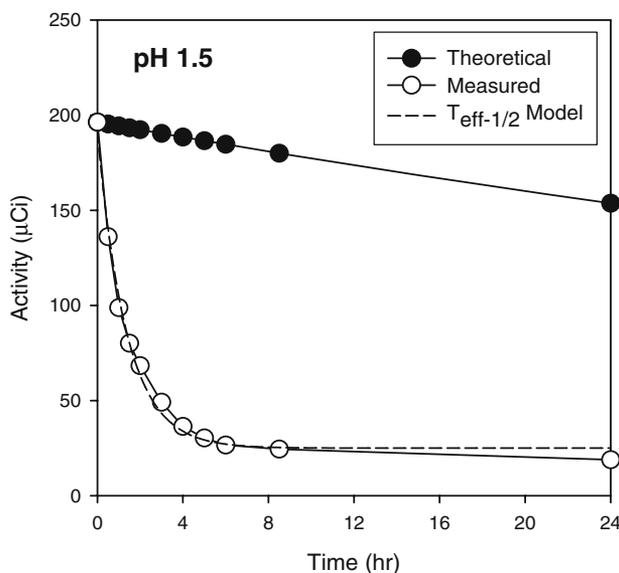
**Fig. 3.** Dissolution at pH 1.5 of a GRF with <sup>153</sup>Samarium Oxide powder versus exponential decay modeling of the  $T_{1/2eff}$  effective half life using the exponential decay model,  $A = C + A_0 e^{-\left(\frac{0.693}{T_{1/2eff}} t\right)}$ , where  $A$  indicates the activity,  $A_0$  is the initial activity,  $T_{1/2eff}$  is the effective half-life,  $t$  is the decay time and  $C$  is a constant calculated during curve fitting.
